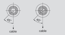
When the shaft marking is set off by 45° from the cable outlet, the output signal is at the start position (min. voltage or min. current). Exception: When using a RSC with 30° active travel, the above position of shaft mar-
