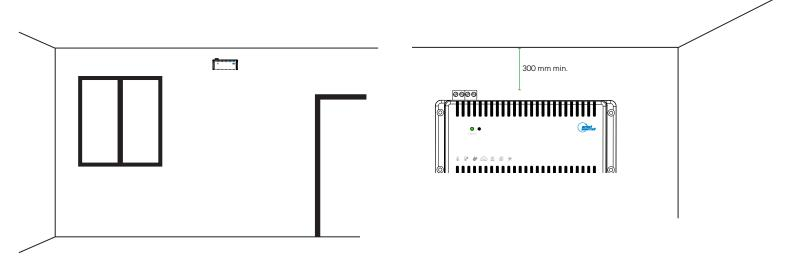
Do not place the device in direct sunlight. There is a risk of the device being heated by the Sun and thus measurement being inaccurate. Do not place the device in an area with the possibility of sudden changes in the air flow. Measured values can be affected and measurement distorted. DANGER OF INCORRECT MEASUREMENT
