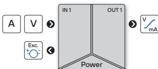
The OMX 39 model series are low-price and simple analog transmitters with mounting on a 35 mm wide DIN rail.
