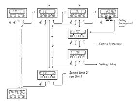
Limit values can be continuously adjusted within the entire measuring range. The switch will occur at the moment when the preset value is reached and exceeded (the relay function can be adjusted). Hysteresis is adjustable in 100% of the measuring range and it informs about the difference by which
