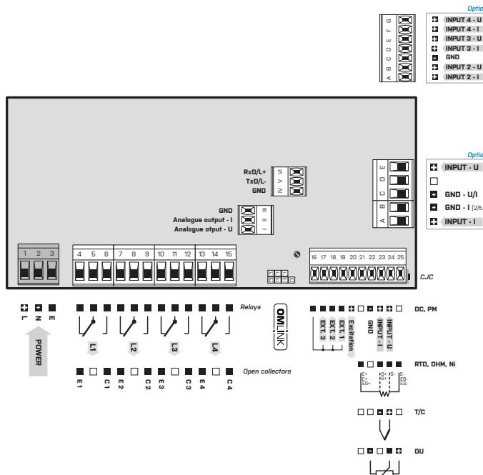
\*GND (Input + Option A) is galvanically connected with inputs EXT. and the OM Link connector
