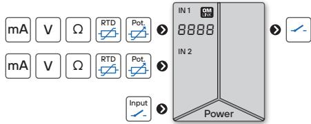
The OMB 200/300/500UNI model series are simple bargraphs designed for maximum efficiency and user comfort while maintaining their favourable price. Type OMB 502UNI is a multifunction instrument with the option of configuration for 5 various input options, easily configurable in the instrument menu.
