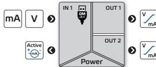
The OMX 200 model series are digital DIN rail mounted trasmitterss housed in an enclosure only 12.5 mm wide.
