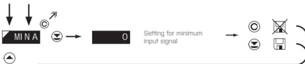
**MIN A** **Setting display projection for minimum value of input signal**
