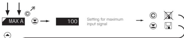
**MAX A** Setting display projection for maximum value of input signal
