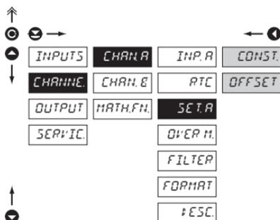
**SET.A** Setting the basic parameters of channel A
