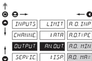
**AN. OUT** Setting the range of the analog output
