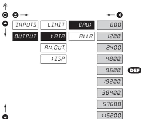
**DATA** Setting the data output rate (baud)
