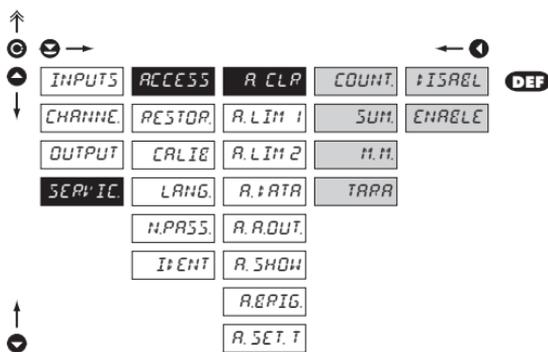
**R.CLR** Authorization for resetting the internal values of the instrument to zero
