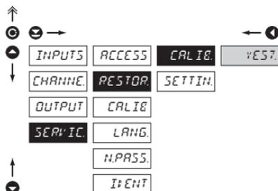
**RESTOR.** Return to manufacture calibration and instrument setting
