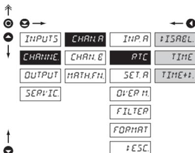
**RTC** Setting the RTC circuit - time backup
