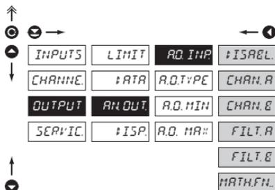
**RO.INP** Setting the input „quantity“ for evaluation of the analog output
