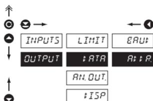
**R: R.** Setting the instrument address
