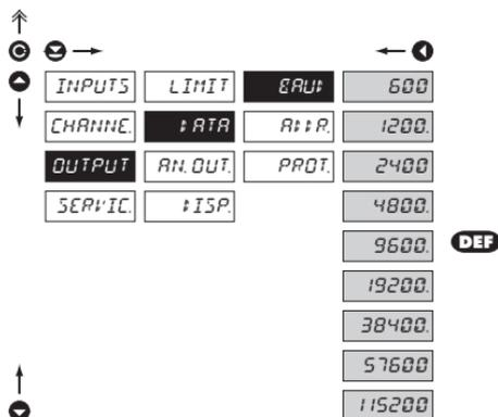
**BAUD** Setting the rate of data output (baud)
