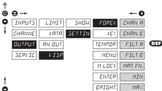
**FOREV.** Selection of values for permanent projection on the instrument display
