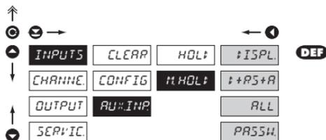
**M.HOLD** Setting the auxiliary input - the HOLD function
