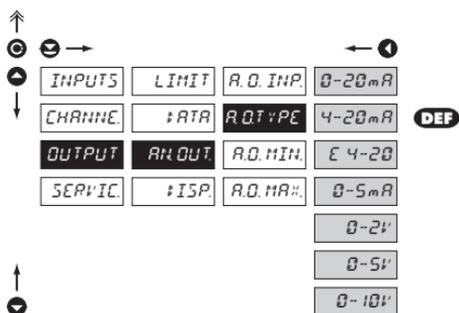
**R.D. TYPE** Setting the type of analog output
