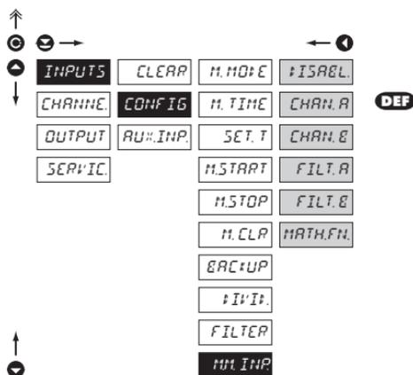
**MM INP** Setting the input „quantity“ for evaluation of the min/max. value
