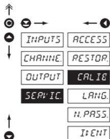
**CALIB.** Instrument calibration
