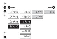
when "C. MIN" is displayed, move the potentiometer traveller to the required minimum position and confirm by "Enter", calibration is confirmed by "YES"
