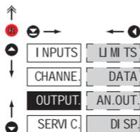
In this menu it is possible to set parameters of the instrument output signals
