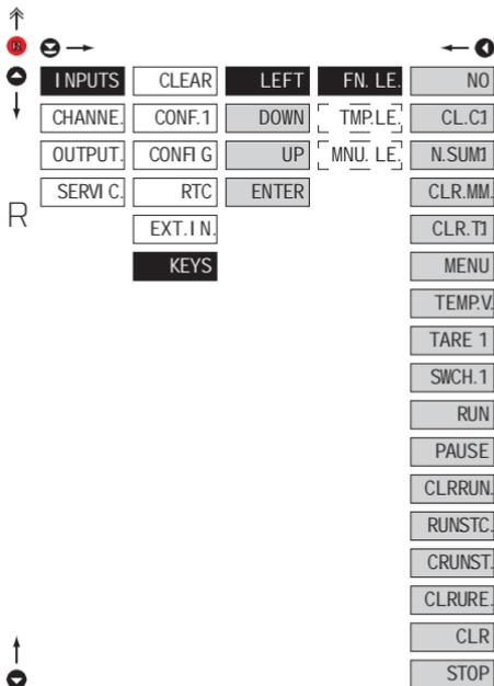
**FN. LE.** Assigning further functions to instrument keys
