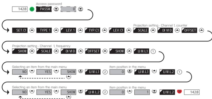
The result of this setting is that when the **R** button is pressed, the display will read „LIM L.1“. By pressing **☺** button you confirm your selection and then you can set the desired limit value, or by pressing the **☺** button you can go to setting of „LIM. L.2“ where you can proceed identically as with Limit one.
