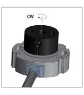
When the indicator of the position marker is pointing towards the cable, the sensor output is near the electrical center position.
