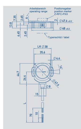
When the shaft marking is pointing to cable, the sensor is located in electrical center position.
