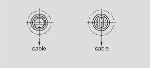
When the shaft marking is pointing to cable, the sensor is located in an electrical center position.
