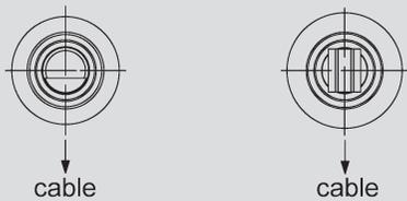
When the shaft marking is pointing to cable, the sensor is located in an electrical center position.
