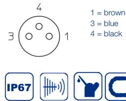
**M8x1 Mating female connector, 3-pin, straight, with molded cable, shielded, IP67, open ended**
