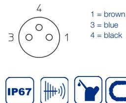
**M8x1 Mating female connector, 3-pin, angled, with molded cable, shielded, IP67, open ended**
